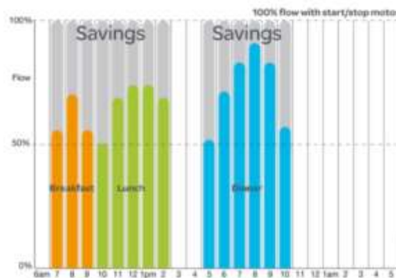
Figure 19. Savings with use of VSD on kitchen hoods 40
